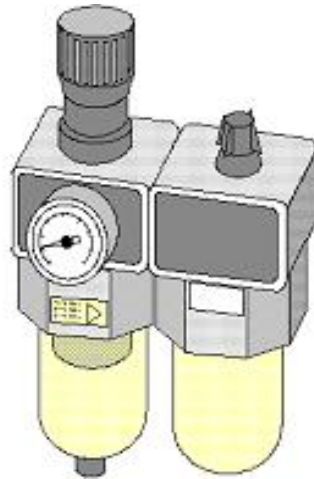
Figure 10.11. Compressed Air Service Unit
